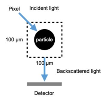
Figure 1. Schematic of the hyperspectral infrared (HSRI) detection setup. A cubic pixel volume  $(100 \times 100 \times 100 \, \mu m)$  receives diffuse incident light, which interacts with embedded particles and is backscattered toward a detector. This geometry models retinal tissue interrogation and underlies the particle count and volume fraction calculations in this appendix.
