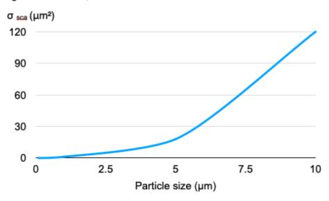
**Figure 2. Scattering Cross-Section vs Particle Size.** Scattering cross-section ( $\sigma_{SCa}$ ) of polystyrene (PS) particles as a function of particle radius at  $\lambda = 500$  nm. The curve illustrates the nonlinear increase in  $\sigma_{SCa}$  with particle size, ranging from 0.012 μm<sup>2</sup> for 10 μm particles, underpinning the enhanced detectability of microplastics compared to nanoplastics.
