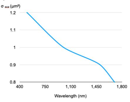
Figure 3. Scattering Cross-Section vs Wavelength. Scattering cross-section ( $\sigma_{SCa}$ ) of 1 µm polystyrene (PS) particles across wavelengths from 500 nm to 1700 nm. The curve shows a modest decline in  $\sigma_{SCa}$ , from 1.2 µm² at 500 nm to 0.8 µm² at 1700 nm, consistent with reduced scattering in the shortwave infrared (SWIR) region. These values are interpolated approximations used to visualize wavelength-dependent sensitivity
