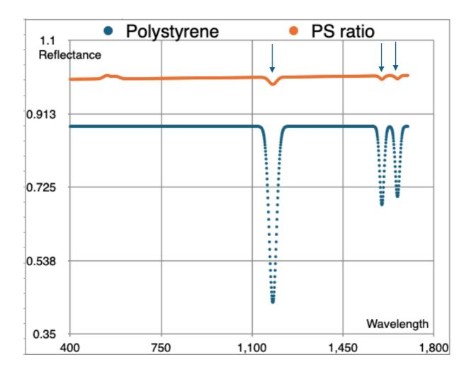
**Figure 3. Detection of Polystyrene Characteristic Absorption.** The normalized PS Ratio signal shows a distinct inflection (arrow) at the same wavelength as the major absorption feature of pure polystyrene. The attenuated amplitude of the feature in the ratio signal is expected when detecting a trace component (3%) within a dominant biological matrix. This visual alignment, combined with strong statistical correlation (r=0.65), illustrates partial recovery of the plastic spectral fingerprint.
